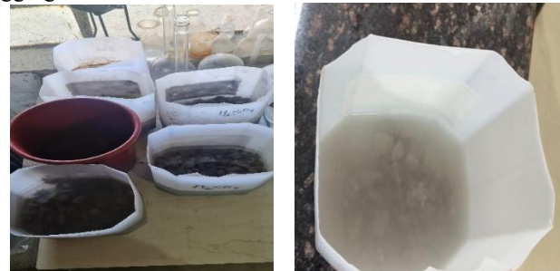
Figure 1 Chemical Reaction Between RCA and Acids
