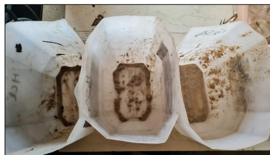
Figure 2 Impurities Left Illustrating the Removal of Adhered Mortar From RCA
