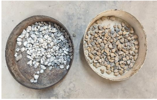
Figure 3 Chemically Treated RCA after 48 hours: H 2 SO 4 (Left Pan), HCl (Right Pan)
