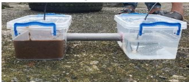
[Fig.4: A Setup of the Dual Chamber MFC Showing the Anode and Cathode Chambers and Proton Exchange Membrane (Salt Bridge)]
