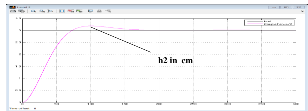
Fig 12. Response of Second Tank using PID
