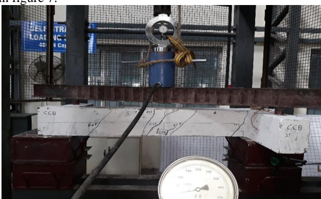
Figure 7 RCC Torsional Beam Testing Arrangements
