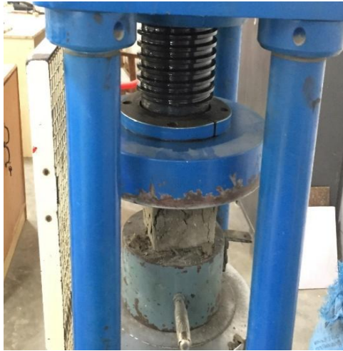
Figure 3 Compressive Strength Test
