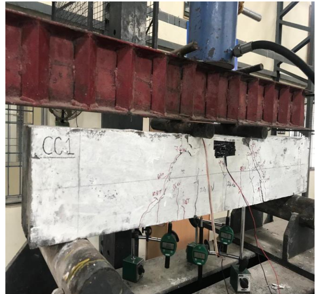
Figure 5 RCC Flexural Beam Testing Arrangements
